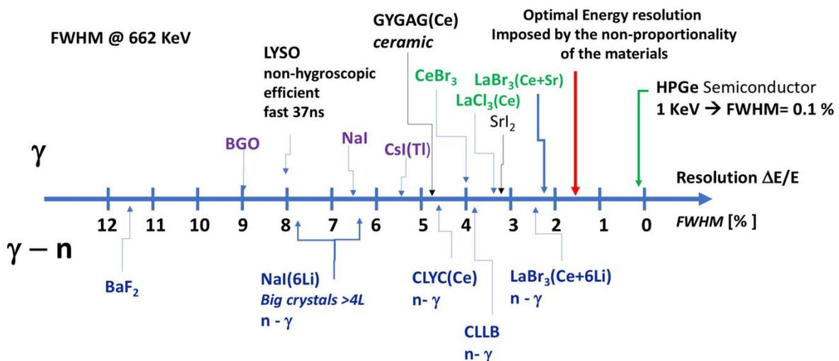
Figure 1: Existing high-resolution scintillator materials ordered according to the energy resolution obtained: FWHM as DE/E in % at 662 keV.
