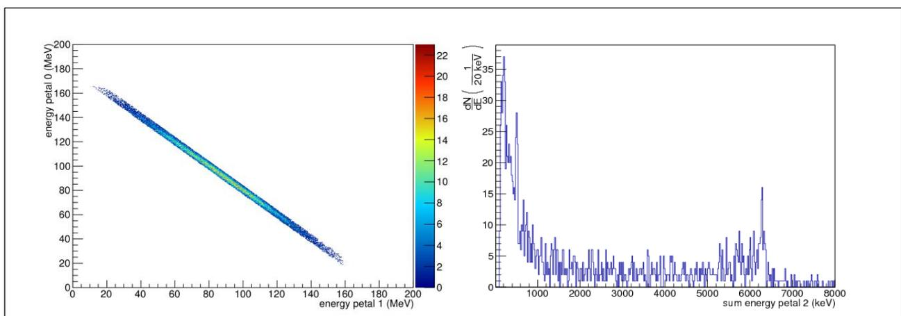
Figure 6. Event selection on the particle energy sum indicating the first excited state (left) and corresponding coincident gamma ray spectrum detected in petal 2 (right). Clearly, the expected line at 6.3MeV and its single and double escape peak dominate the spectrum.
