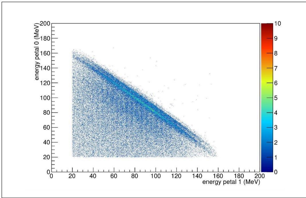
Figure 5. Correlation of the energy depositions in the petals 0 and 1 mounted opposite to each other. Here multiple anti correlations are observed in the data. As we know from kinematic simulation of a  $^{16}\text{O}(p,2p)$  reaction two lines corresponding to the ground state and first  $3/2^-$  excited state of the  $^{15}\text{N}$  nucleus dominate the spectrum. The elastic proton - proton scattering was suppressed by an opening angle cut.
