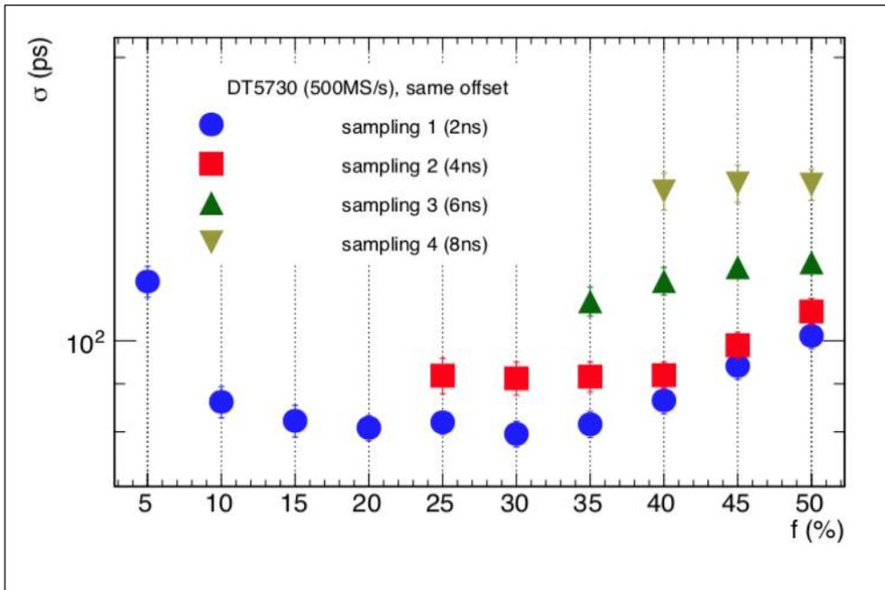
Figure 2. Sigma from the Gaussian fit to the time differences obtained for the DT5730 versus fraction of different samplings. The fraction f is a parameter of the algorithm which is used to determine the time of each signal. The sampling describes how much the signal sampling period was increased, to simulate a slower ADC.
