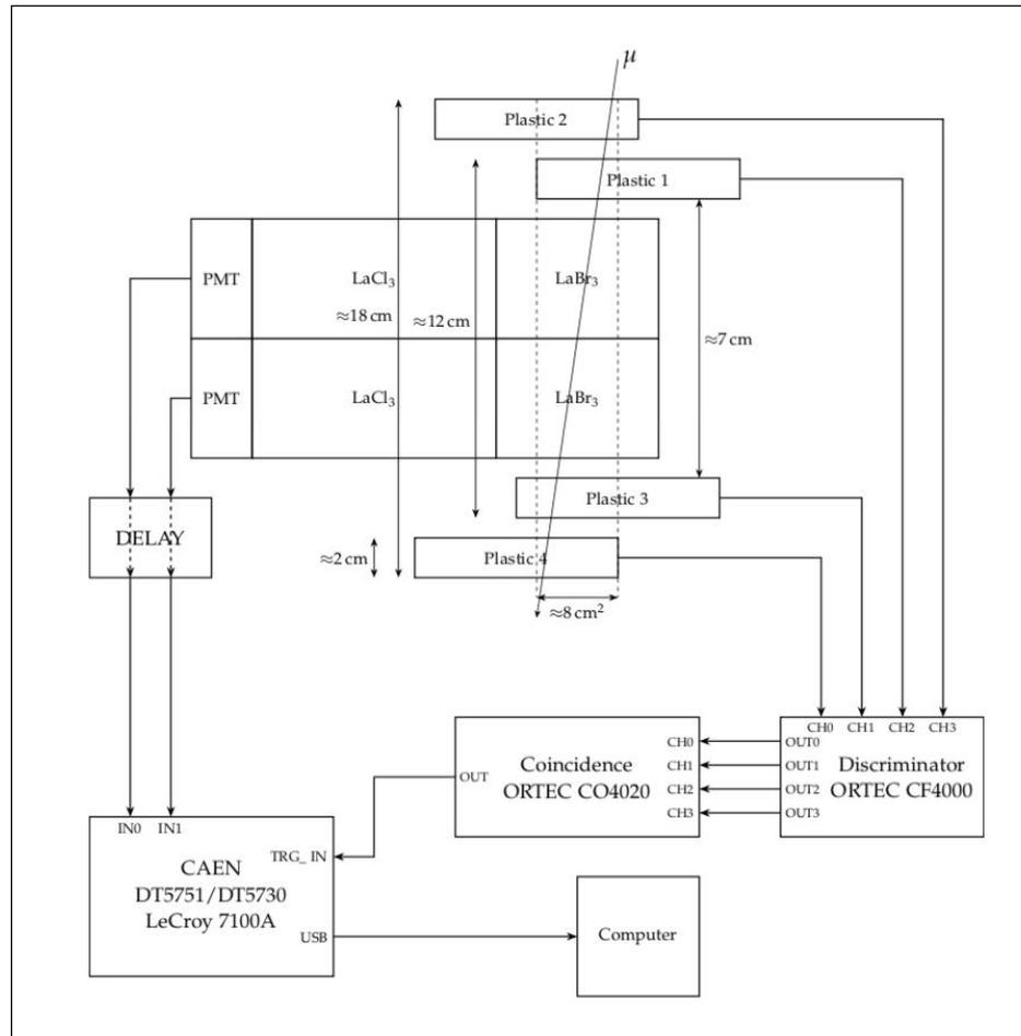
Figure 1. Schematic view of the setup for detecting and tracking cosmic muons passing through the CEPA4 demonstrator.
