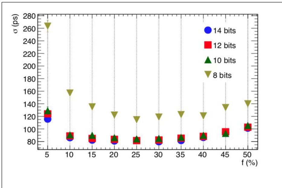
Figure 3. Sigma from Gaussian fit to the time differences obtained for the DT5730 versus the fraction f for different bit resolutions.
