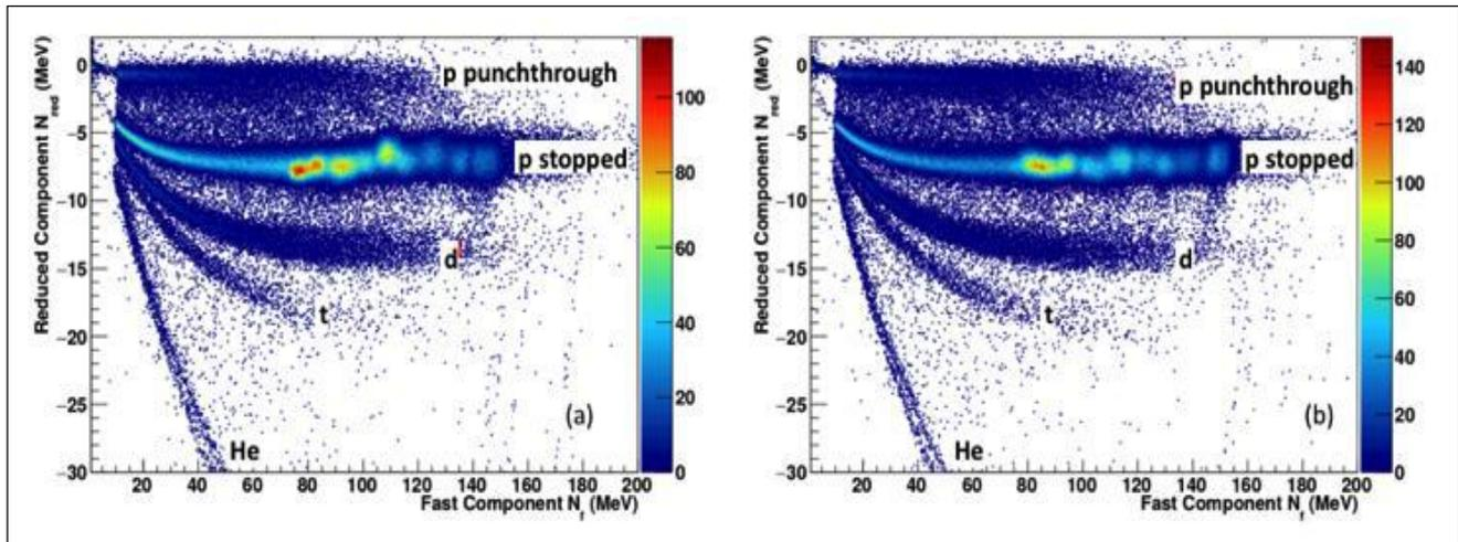
Figure 7. The figures shows the PID plot in reduced representation, as explained in the text above. In both petals the branches of stopped and punch through protons are clearly separated down to an artificial threshold visible at 10 MeV. Furthermore, deuterons, tritons, and He are identified as well.
