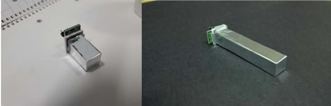
Figure 2: Left: Phoswich unit formed by GAGG  $1 \times 1 \times 1 \text{ cm}^3$  + CsI(Tl)  $1 \times 1 \times 1 \text{ cm}^3$ . Right: Phoswich unit formed by GAGG  $1 \times 1 \times 3 \text{ cm}^3$  + CsI(Tl)  $1 \times 1 \times 1 \text{ cm}^3$
