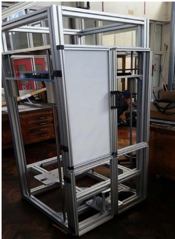
Figure 12: Collimated source enclosure under construction in the UoY workshop (July 2017).
