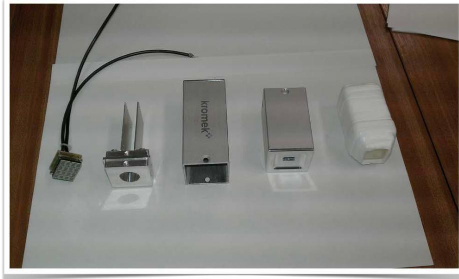
**Figure 1: Hand-held gamma-ray spectrometer based on SiPM/CsI(Tl) combination developed by UoY for Kromek PLC.**
