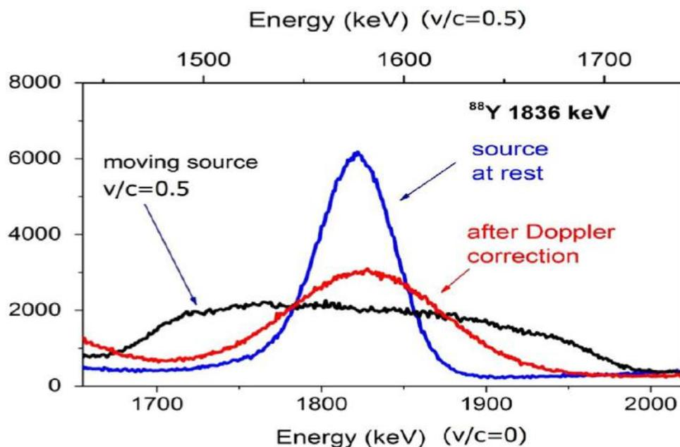
**Figure 4:** The black line shows the measured spectrum of the 1836 keV simulating a source moving with  $v/c = 0.5$ . The energy scale is on the top of the figure. For comparison, the measured original spectrum is also shown (blue line, energy scale on the bottom of the figure). The measured spectrum obtained after Doppler correction (red line) is also plotted. Figure from Ref. [1].
