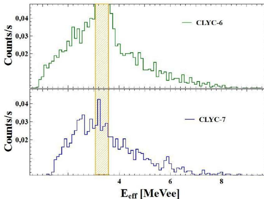
Figure 2. Comparison between the neutron experimental spectra of the two CLYC crystals. Top panel: CLYC-6 measured energy spectrum. The region between 3.1 MeV and 3.6 MeV is completely dominated by the thermal neutron peak (due to the interaction in  $^6\text{Li}$ ). Bottom panel: CLYC-7 measured energy spectrum. Figure is from the ANSRI conference proceedings.
