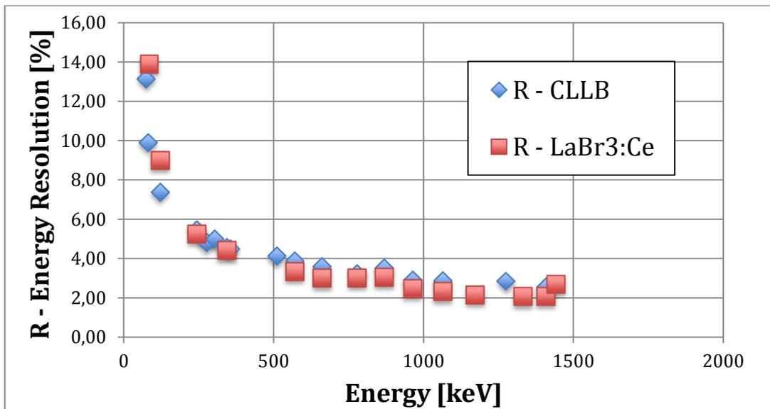
Figure 1. Energy resolution versus energy of gamma-rays measured in CLLB and  $\text{LaBr}_3:\text{Ce}$  crystals.
