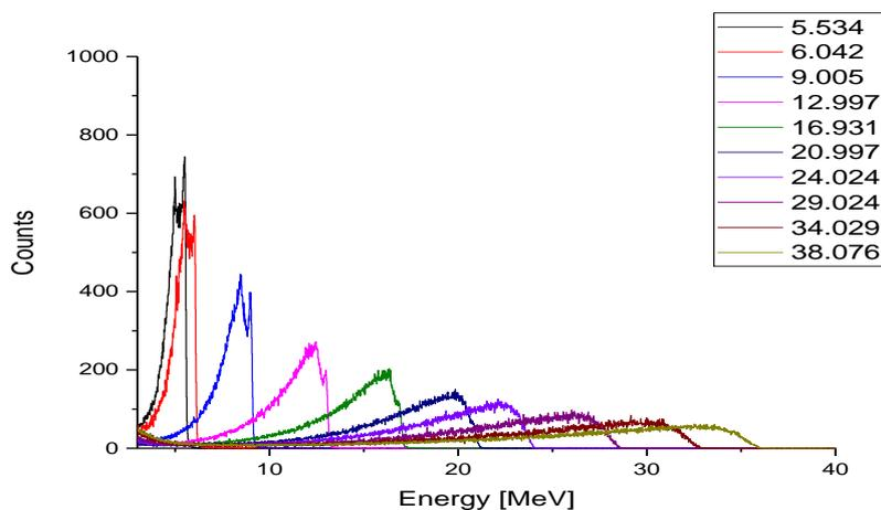
Figure 3. Measured gamma-ray response function with a LaBr<sub>3</sub>:Ce detector from the HECTOR+ array. The inset lists the gamma-ray energies produced by Compton backscattering.
