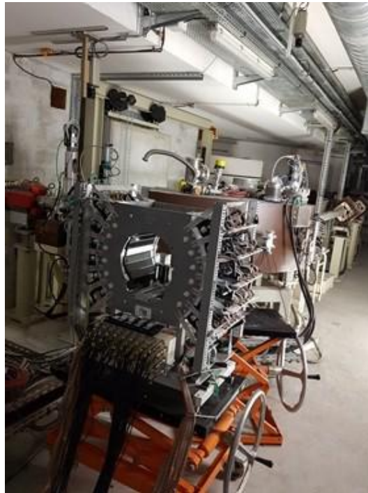
Fig. 29: Large-acceptance pixelated detector demonstrator module installed at the 65 MeV proton Medicyc line of the Centre Antoine Lacassage at Nice.
