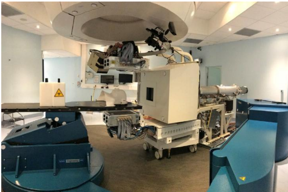
Fig. 23: Picture of the updated version of the INSIDE bi-modal system. The PET heads are visible above and below the treatment bed. The DP is on the upper left side, pointing toward the isocenter.
