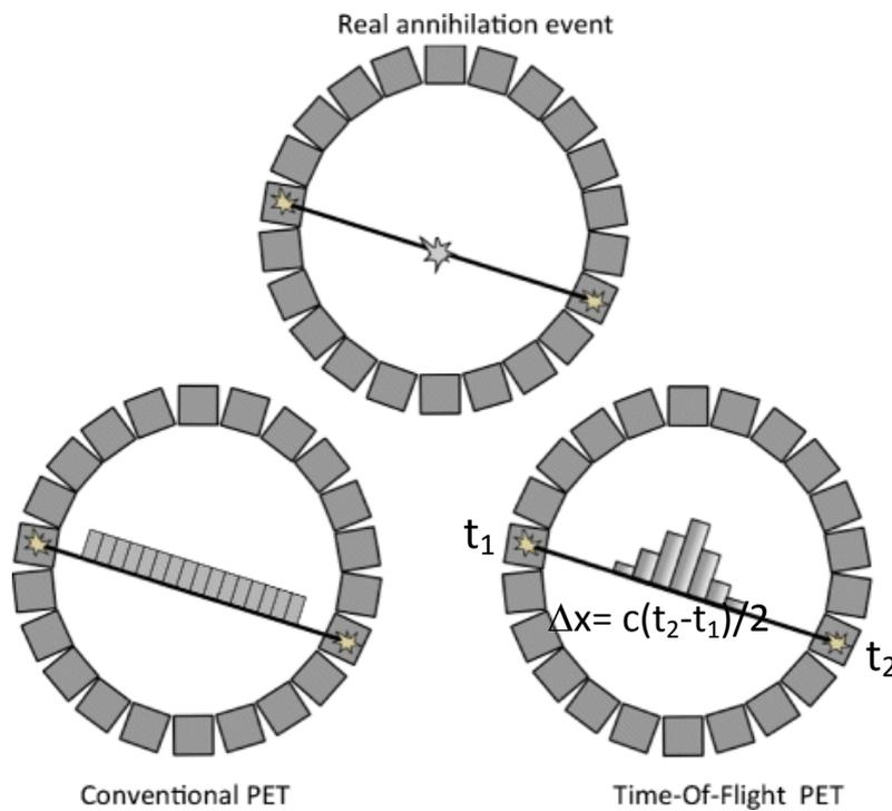
**Fig. 4:** Illustration of PET photon detection principle. With conventional PET, the annihilation event has a uniform probability along the Line of Response (LOR). Time of Flight enables one to reduce the probability along a segment of length  $\Delta x = c\Delta t / 2$ , where  $\Delta t$  is the coincidence timing resolution, and  $c$  the speed of light.
