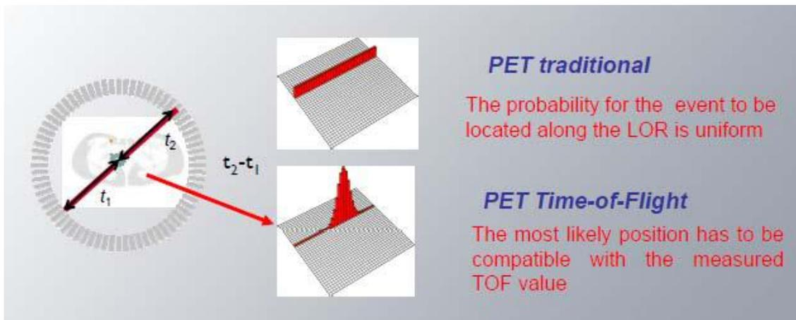
**Figure 9:** Illustration of the principle of time-of-flight PET measurement (ToF-PET), allowing to increase the image contrast.
