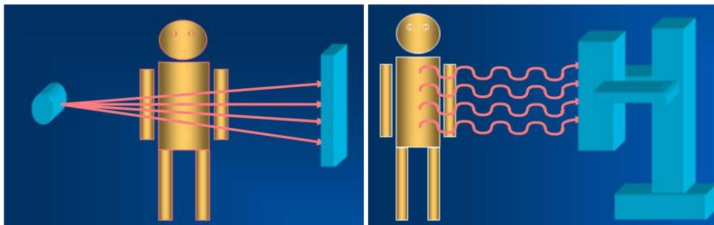
**Figure 7:** Left: Schematic illustration of (X-ray) transmission imaging. Right: Scheme of (photon) emission imaging (as used in PET and SPECT devices)
