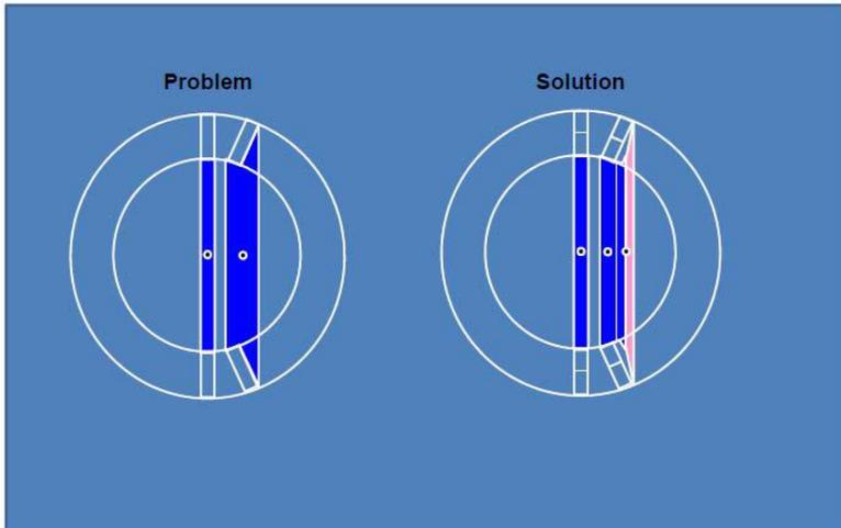
**Figure 8:** Illustration of the ‘depth of interaction (DOI)’ effect in PET photon registering.
