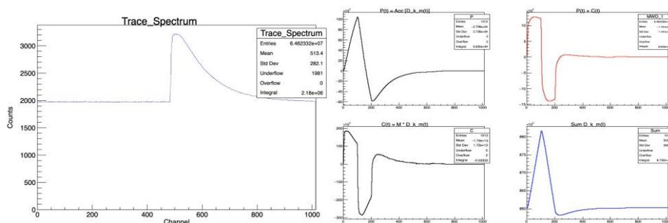
**Figure 3 (Left side) An example of alpha trace signal. (Right side) A trapezoidal filter applied to the signal to extract the energy and time of the alpha particle.**
