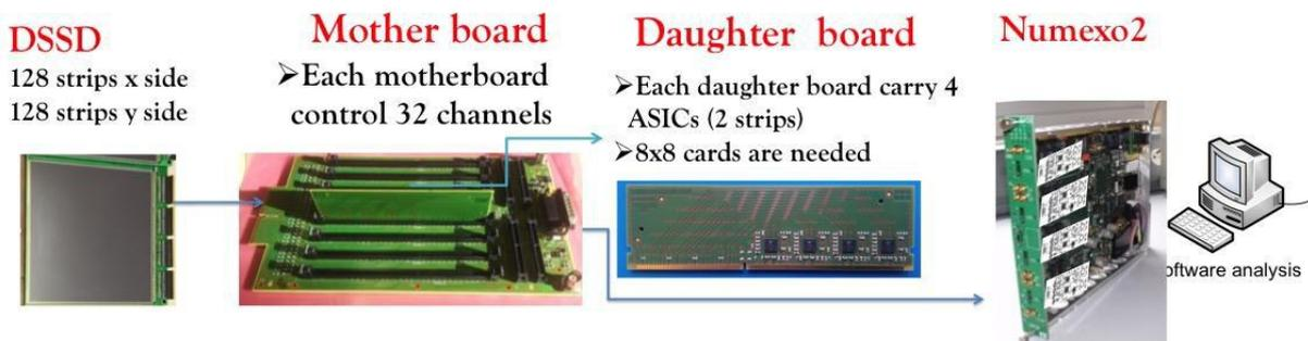
Figure 2 The full electronics chain is shown, where all the components from the motherboard to the daughter board hosting the Asics are shown.
