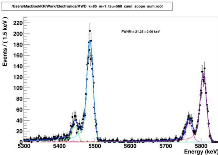
Figure 3 Energy spectrum of triple alpha source Am, Cm , Pu.
