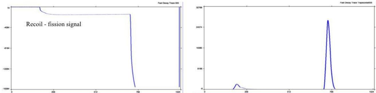
Figure 4 (Left side) Digital signals of recoil followed by a spontaneous fission signals. (Right side) Filtered data in order to extract energy and time of particles hitting the detector.
