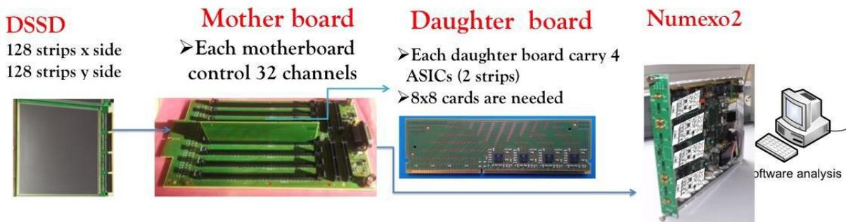
Figure 2 The full electronics chain is shown, where all the components from the motherboard to the daughter board hosting the Asics is shown.
