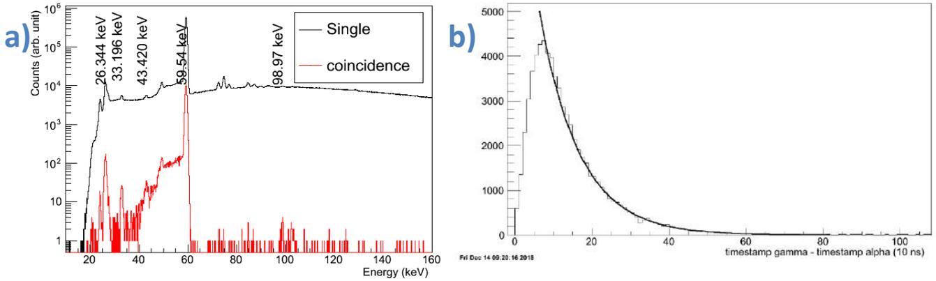
Figure 1 – a) LEPS single and coincidence spectrum - source combination: <sup>241</sup>Am + <sup>60</sup>Co – b) Decay curve: 1<sup>st</sup> 5/2<sup>-</sup> state of <sup>237</sup>Np populated by <sup>241</sup>Am α decay (note the x-axis unit: 10 ns).
