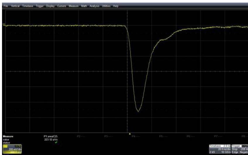
Figure 5. Signal of EJ301 + PMT from oscilloscope LeCroy. Time base is 20 ns/division.
