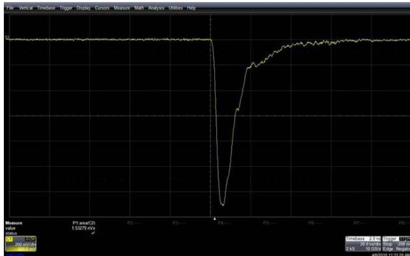
Figure 6. Signal of EJ299 + PMT from oscilloscope LeCroy. Time base is 20 ns/division.
