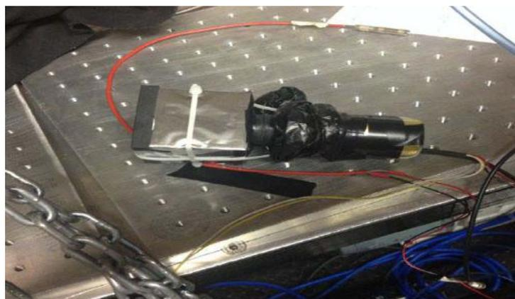
Figure 3. Scintillator EJ299 assembled with phototube.
