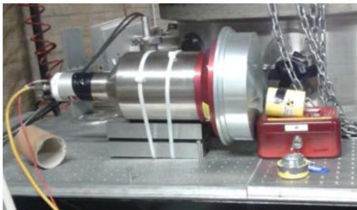
Figure 2. Scintillator EJ301 coupled with phototube.
