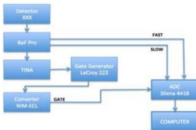
Figure 4. Block diagram of the electronic for the PSD.
