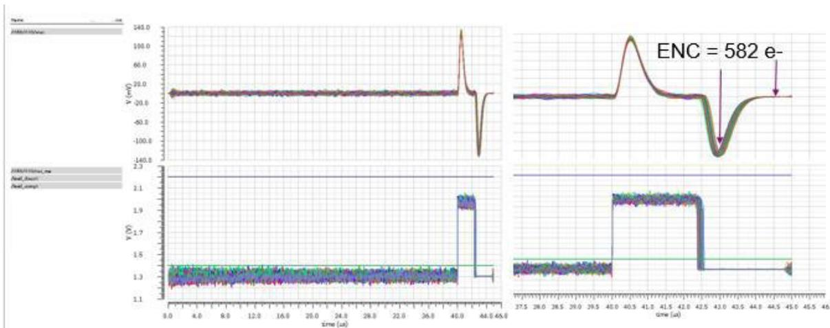
Figure 8 : transient noise analysis of the High GAIN with 100 runs, Noise Fmax = 10 MHz, Fmin = 100, Noise seed = 1 and noise scale = 100 with Cd = 60 pF, input MOS 8 mm
