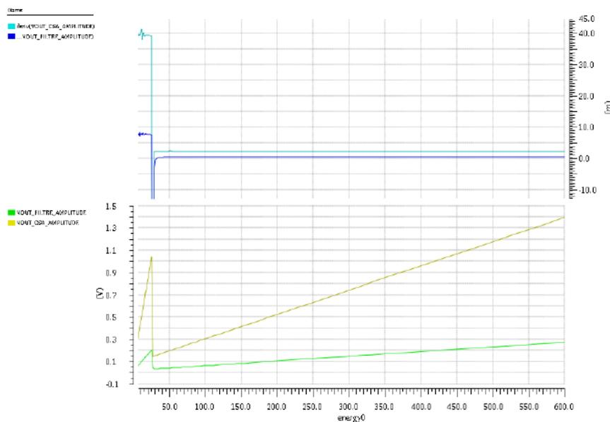
Figure 7 : the linearity of the CSA for different energies [1 – 600 MeV] Cd = 200 pF, V\_Trigger = 1,31 V and V\_LG = 2,3 V
