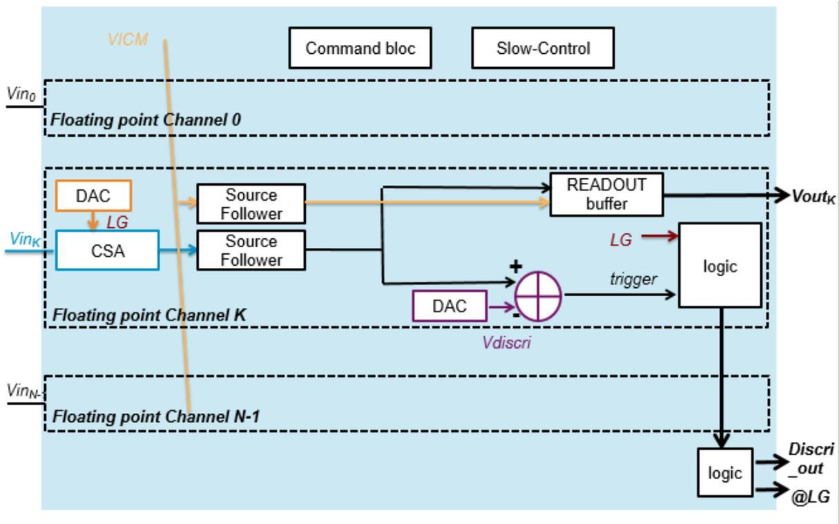
Figure 5 : global architecture of the multi-channel FPCSA V2 chip
