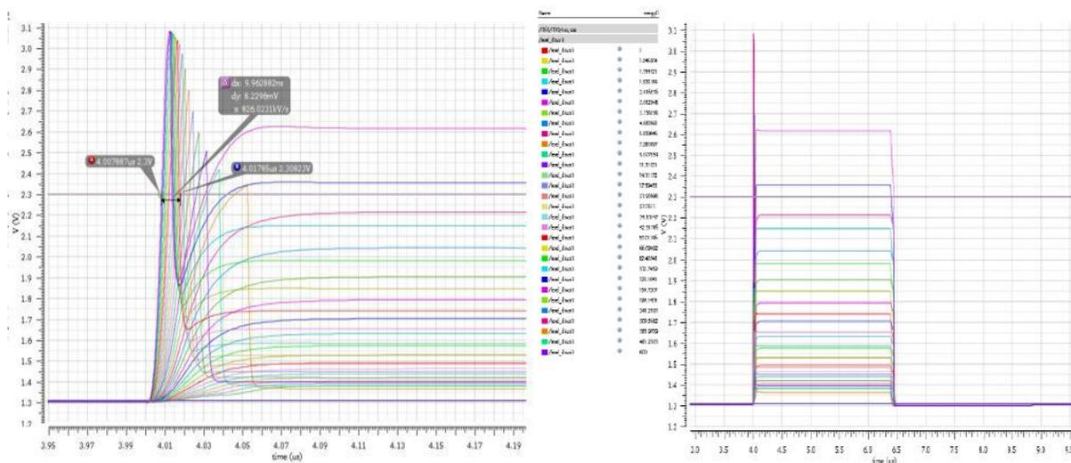
Figure 6 : Transient output signal of the CSA for different energies [1 – 600 MeV] with Cd = 200 pF, V\_Trigger = 1,31 V and V\_LG = 2,3 V
