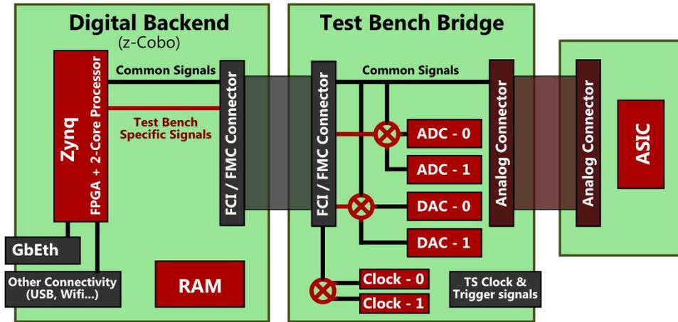
Figure 2: Test bench hardware setup.
