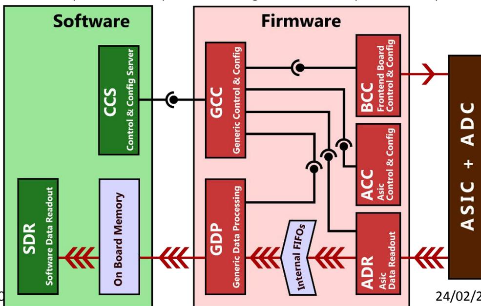
Figure 1: Main firmware & software components.
