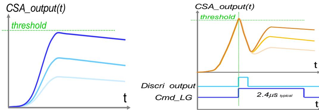
Figure 4 : CSA output for low energy events (left) and for high energy events (right)
