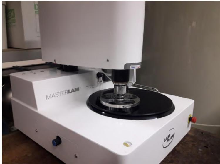
Figure 1: Metallographic polishing (MP) device.
