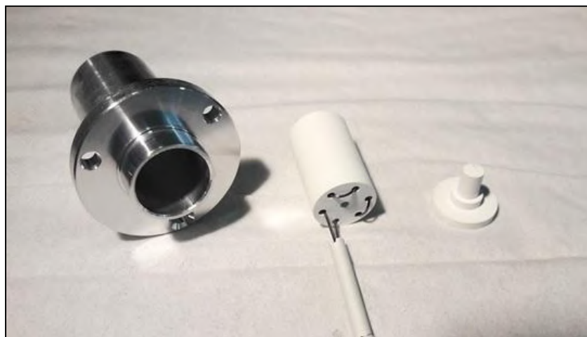
Figure 15: Heater assembly for reactants with low boiling point (CERN). From left to right: Aluminium case, heating cartridge: boron nitride insulating the tantalum heating wires and containing the sulphur powder, plug.
