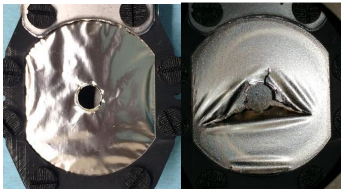
Figure 9: Image of the nickel foil installed on its graphite frame before (left) and after (right) the heating period.
