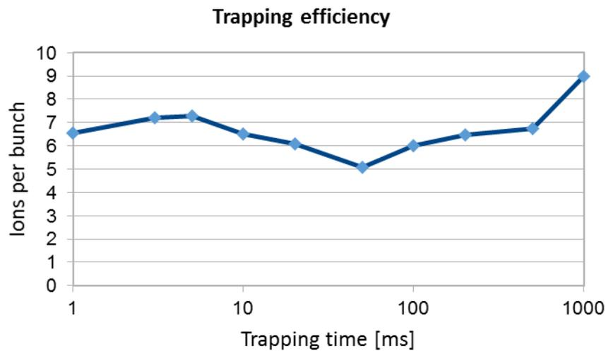
**Figure 8:** Trapping efficiency test for  ${}^7\text{Li}^{1+}$  ions with a lower ion energy (30 eV) showed that there is no significant losses at longer trapping duration, contrary to what was seen for ion energies of 70 eV (see Figure 3).
