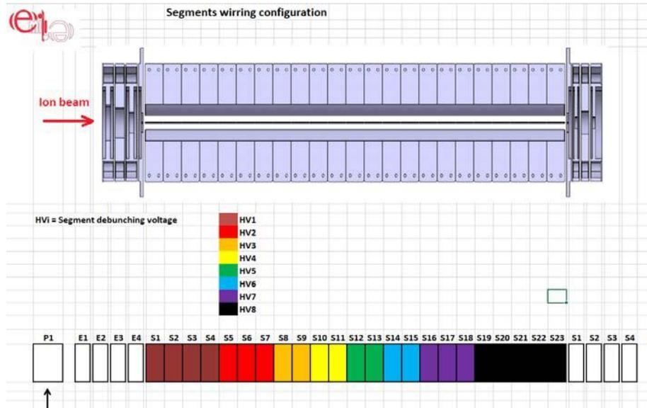
**Figure 3:** The grouping of the 23 internal electrodes of the debuncher used in the tests (December 2017 and January 2018 test – see the text for details). There are 8 groups of DC segment, each with a time-varying HVx potential.
