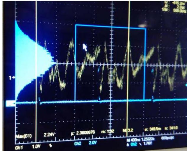
**Figure 5:** HV platform oscillations induced by the arbitrary waveform generator superimposed with the the inherent ripple from the main high voltage power supply. On the x-axis one major unit corresponds to 400 ns and on the y-axes 1 V.
