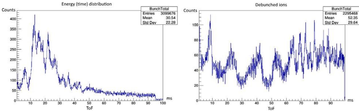
**Figure 14:** Second 100 ms debunching run: The axial momentum distribution scanned by linear ramp potential during the trapping period of 100 ms (left-hand). The beam extracted by the inverse integral function (right-hand).
