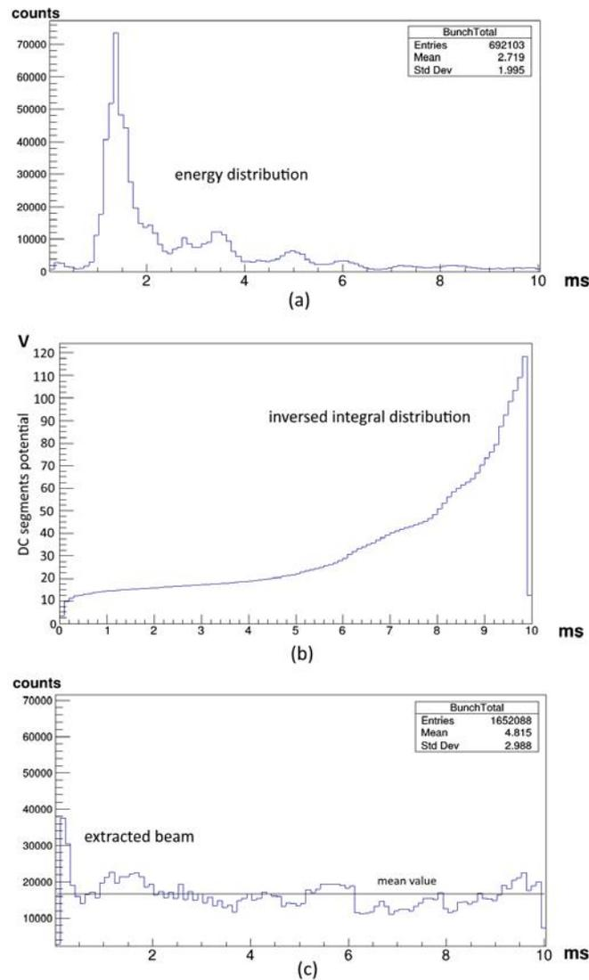
**Figure 11:** (a) The axial momentum distribution of  ${}^7\text{Li}^{1+}$  ( $E=30$  eV) measured by applying a linear ramp potential to the ejecting DC electrodes; obtained from step 2 in Figure 7. (b) The inverse integral distribution (step 5 in Figure 7) and (c) the extracted beam, which exhibits a quite uniform intensity in time.
