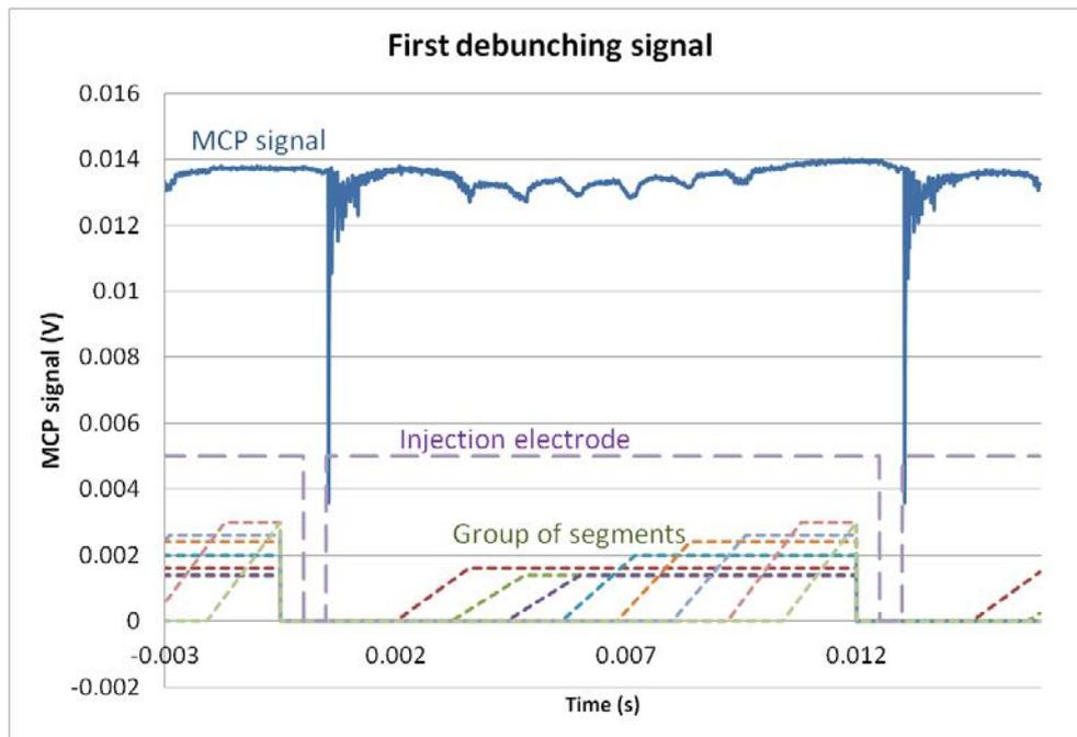
**Figure 2:** Debunching sequence. The dashed lines represents the voltages applied to the successive group of segments (see Figure 3) of the trap and the injection electrode (in arbitrary units). The Micro-Channel Plate (MCP) signal of detected Cs ions, as observed on the oscilloscope, is shown as the solid blue line. The signal polarization is negative, with a base level of about 14 mV.
