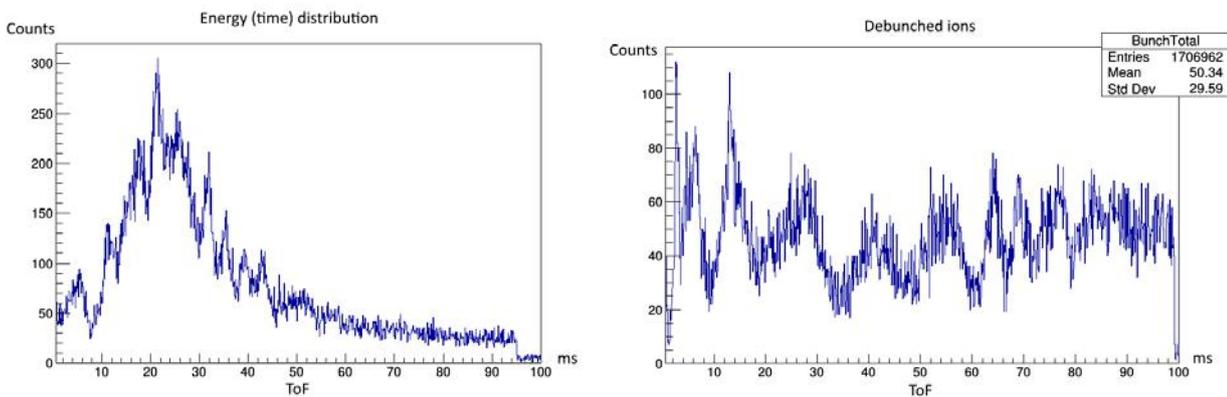
**Figure 13:** First 100 ms debunching run: The axial momentum distribution scanned by linear ramp potential during the trapping period of 100 ms (left-hand). The beam extracted by the inverse integral function (right-hand).
