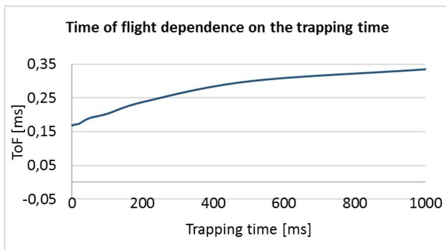
**Figure 9:** Time-of-flight as a function of the trapping time. The average ion velocity changes by a factor 2 between short trapping times (around 10 ms) and a 1 s trapping time.
