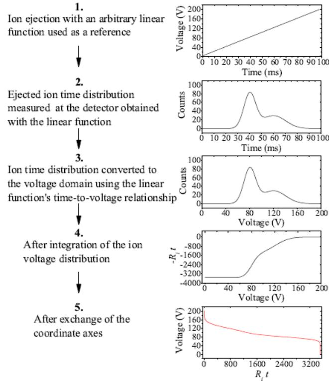
**Figure 7:** Method adapted from Lapierre [5].  $R_i$  is a constant rate of ion extraction (see [5] for details) and the  $R_i t$  corresponds to the lowering rate of the exit DC gate. Instead of lowering the potential of the exit gate, we increased the potential of the inner DC electrodes inside the trap to produce the debunched beam.
