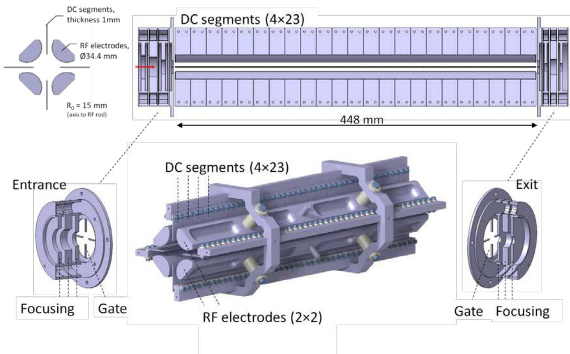
**Figure 1.** Drawings of the debuncher prototype and its main parts. Entrance and exit gate electrodes have X-shaped fingertips in order to increase the transmission efficiency.
