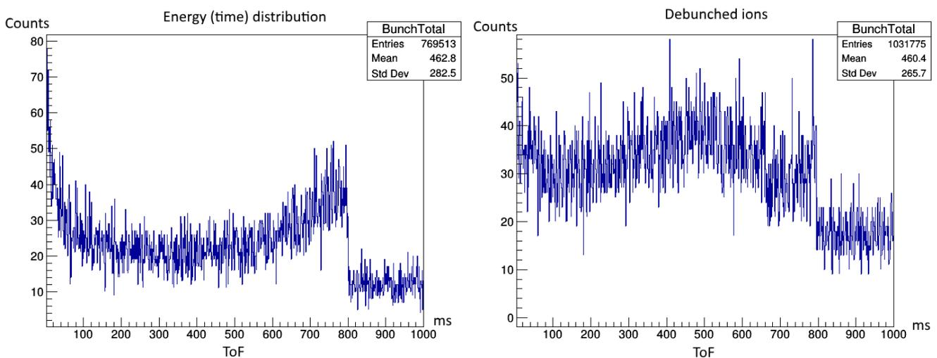
**Figure 15:** 800 ms debunching: The axial momentum distribution scanned by linear ramp potential during the trapping period of 800 ms (left-hand). The beam extracted by the inverse function (right-hand).
