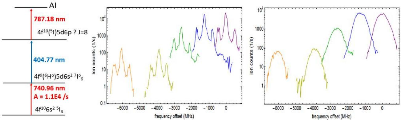
Figure 3: Isotope shifts of the 741-nm ground state transition in stable, zero-spin dysprosium isotopes. The unstabilized laser operation leads to strong frequency jitter and visible side bands at  $\sim 450$  MHz, suppressed by approximately one order of magnitude (left). By fast scanning of a piezo-mounted cavity mirror a stable linewidth of  $\sim 600$  MHz is achieved (right).
