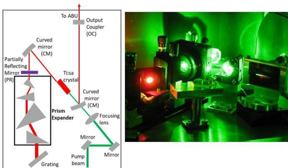
Figure 1: (Left) schematic of the self-seeding grating-based Ti:sapphire laser. (Right), photograph of the standard grating-based Ti:sapphire laser in use.
