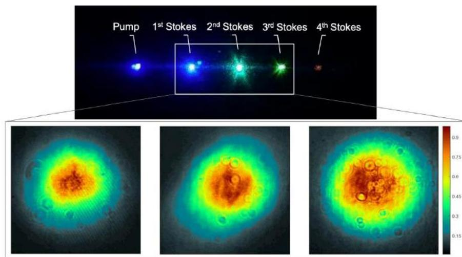
*Figure 6:* Different Stokes orders which can be generated with laser light at 450 nm (top) and the corresponding laser beam profiles (bottom). A more detailed investigation into the cascading effect was launched and details will be published in [3].
