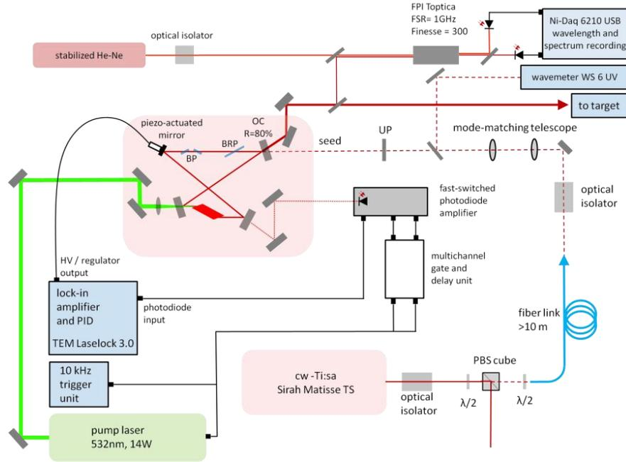
Figure 2: Overview of the setup of the injection-locked Ti:sapphire laser system at JYFL [1].
