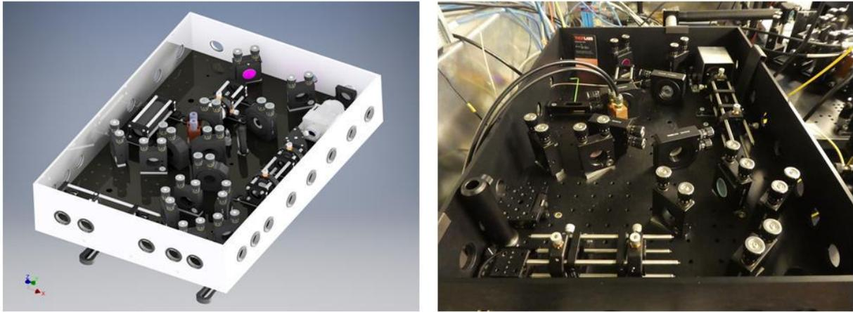
Figure 4: (Left) 3-D design of a new injection-locked Ti:sapphire laser cavity for use at the future MARA-LEB facility. (Right) Photo of the finished laser resonator.
