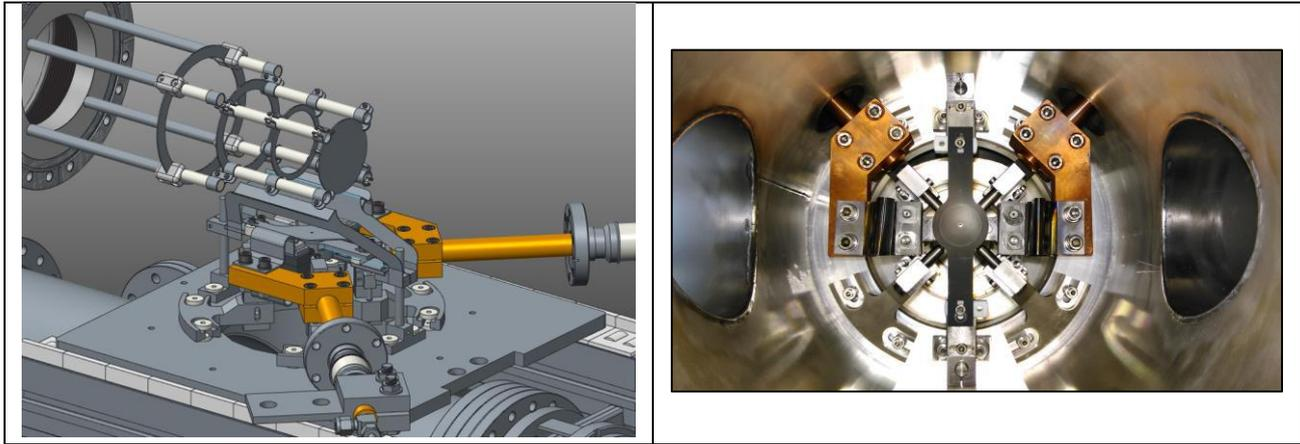
Figure 7: 3D drawings of the evaporation oven (left) and its preliminary installation (right).
