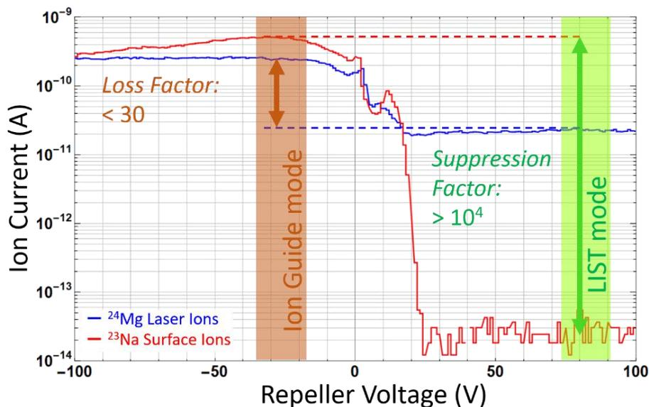
Figure 2: Ion currents of laser-ionised  $^{24}\text{Mg}$  and surface-ionised  $^{23}\text{Na}$  versus the repeller voltage measured with the LIST unit used for the IS614 experiment in June 2018 at ISOLDE.
