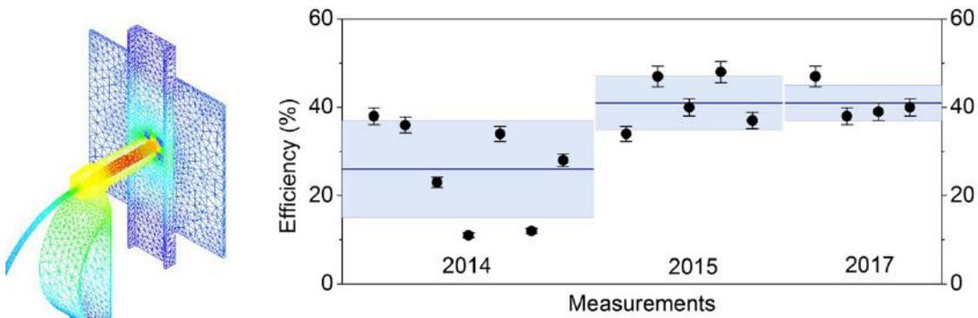
Figure 6: (Left figure) Finite-element simulation of the hot-cavity laser-ion source; (right figure) development of experimental ionisation efficiencies for holmium with reproducibility achieved in recent years (grey range).
