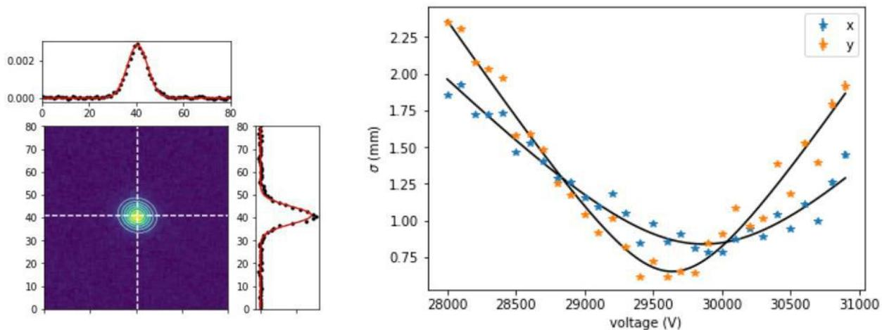
Figure 5: (Left) Image of the beam spot on the phosphor screen recorded by a CCD camera and the corresponding fit of the Gaussian intensity distributions in the vertical and horizontal dimensions. (Right) Spatial width of the beam spots for the vertical and horizontal components as a function of the Einzel lens voltage.
