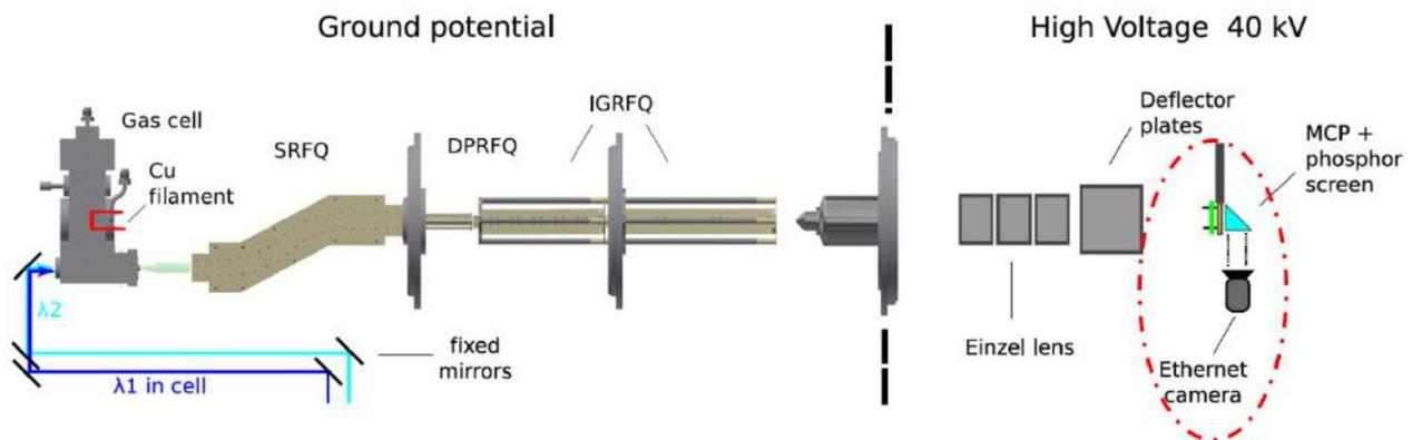
Figure 4: Schematic representation of the IGLIS setup at KU Leuven used to determine the transverse emittance of the ion beam extracted from the RFQ ion guides.
