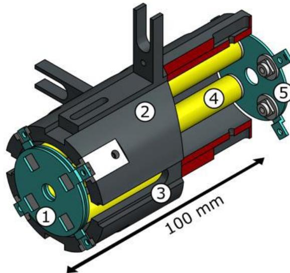
Figure 1: Technical drawing of the newly developed Laser Ion Source and Trap comprising two repelling electrodes (1), housing (2), side cuts for perpendicular illuminations (3), four rods forming the rf-quadrupole structure (4), and exit electrode (5) [1].
