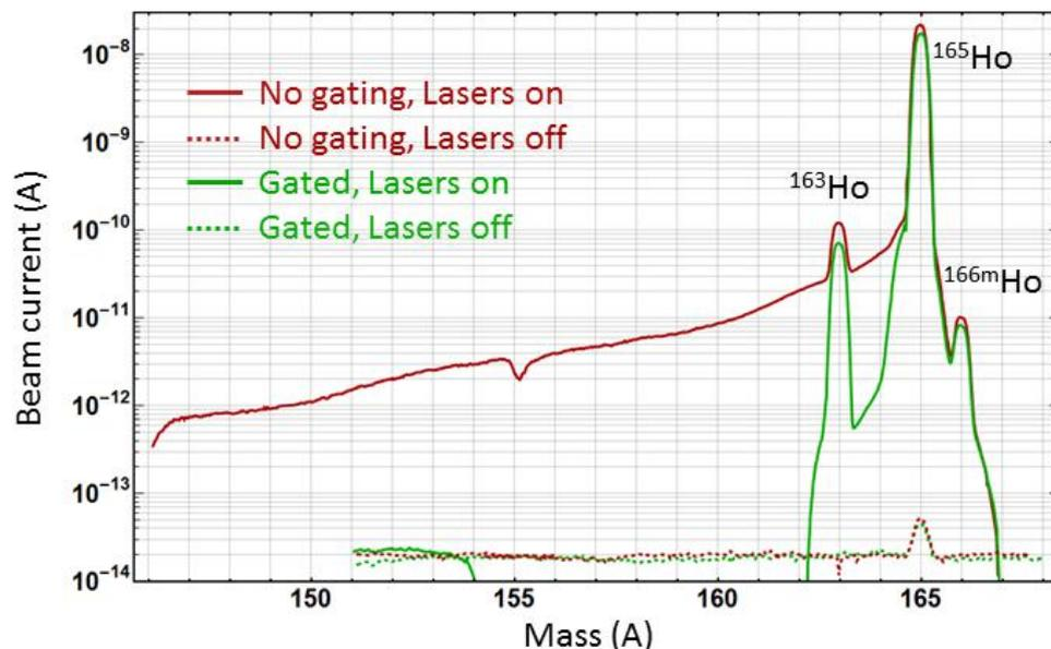
Figure 3: Mass scans in the holmium mass region illustrating the standard operation (red line) and fast ion-beam gating (green line) on a sample of  $^{163,165,166\text{m}}\text{Ho}$ . Non-specific background at the lower mass side stemming from ionisation in the acceleration region is clearly suppressed (dotted lines show negligible surface-ionisation background).
