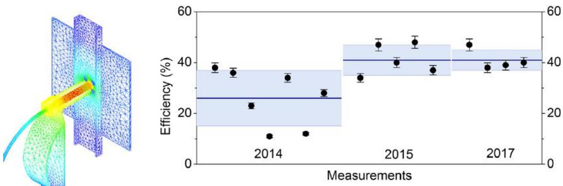
Figure 5: (Left figure) Finite element simulation of the hot cavity laser ion source, (right figure) development of experimental ionization efficiencies for holmium with reproducibility achieved in recent years (grey range).
