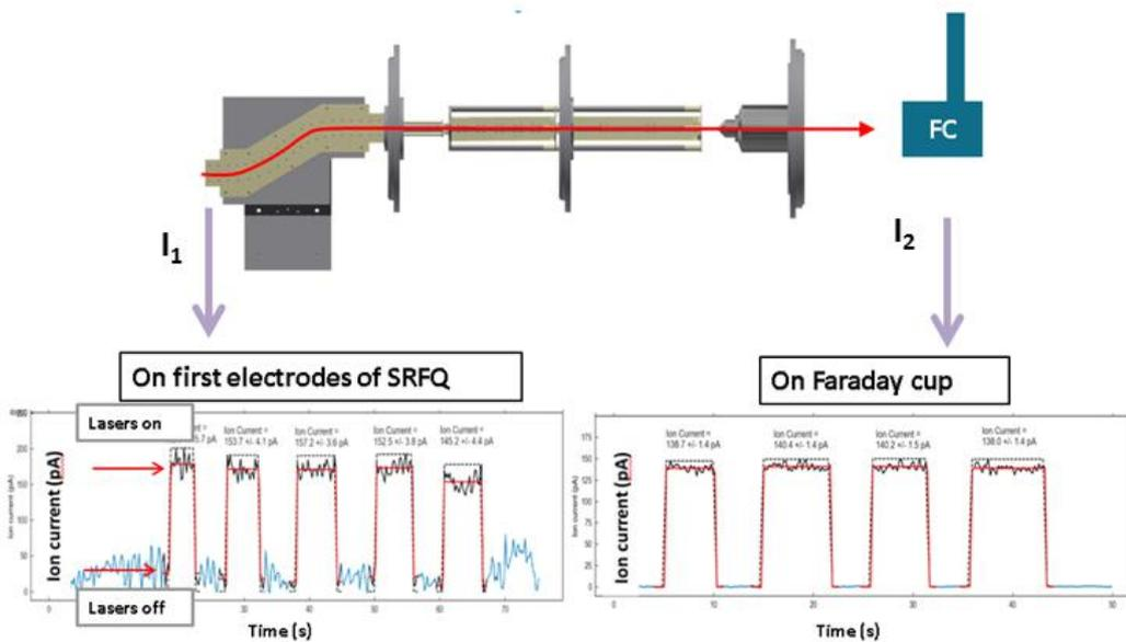
Figure 2: Schematic representation of the HELIOS rf ion guides (S-shaped and linear), installed at KU Leuven. By monitoring the currents  $I_1$  and  $I_2$ , the transmission efficiency of the system can be measured.
