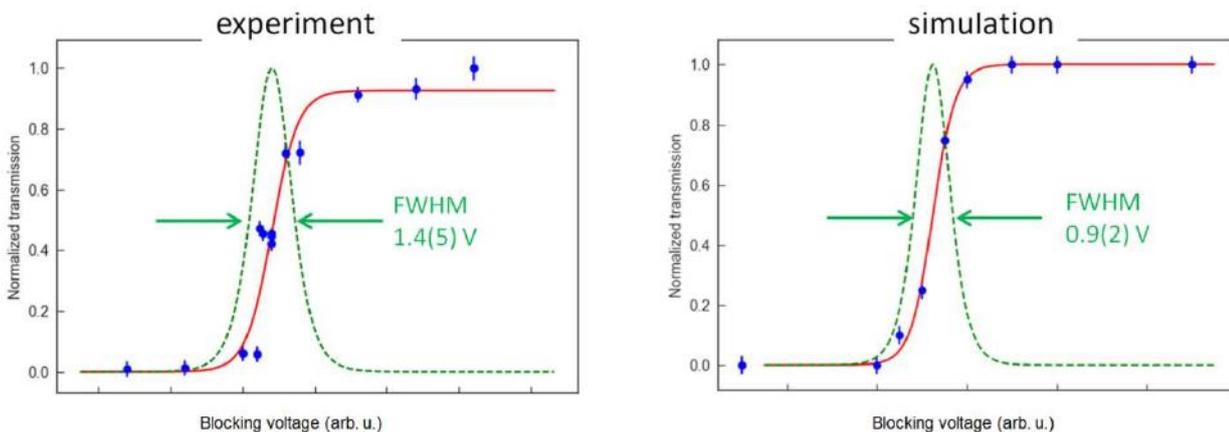
Figure 4: Measurement (left) and simulation (right) results of the longitudinal emittance of the ion beams transported through the RFQ ion guides.
