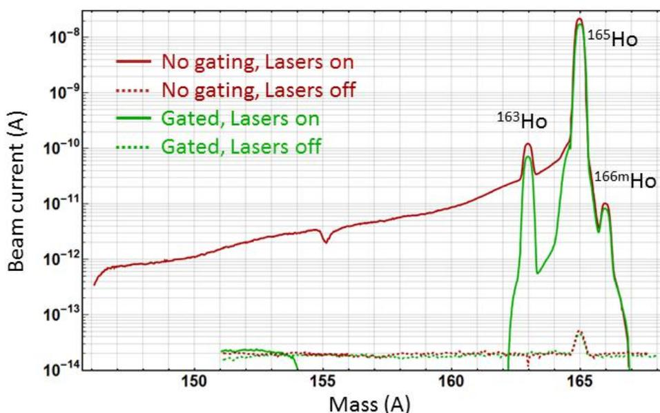
Figure 1: Mass scans in the holmium mass region for comparison between standard operation (red line) and fast ion beam gating (green line) on a sample of  $^{163,165,166\text{m}}\text{Ho}$ . Non-specific background at the lower mass side stemming from ionization in the acceleration region is clearly suppressed (dotted lines show negligible surface ionization background).
