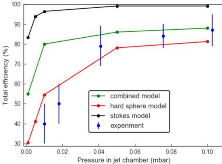
Figure 3: Comparison between the experimental transmission efficiency and different simulations for the radiofrequency ion guides at KU Leuven.
