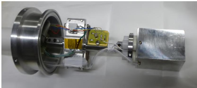
Figure 2.2: Semi-planar crystal placed in a POPTOP type capsule. The assembly and front-end electronics is shown.
