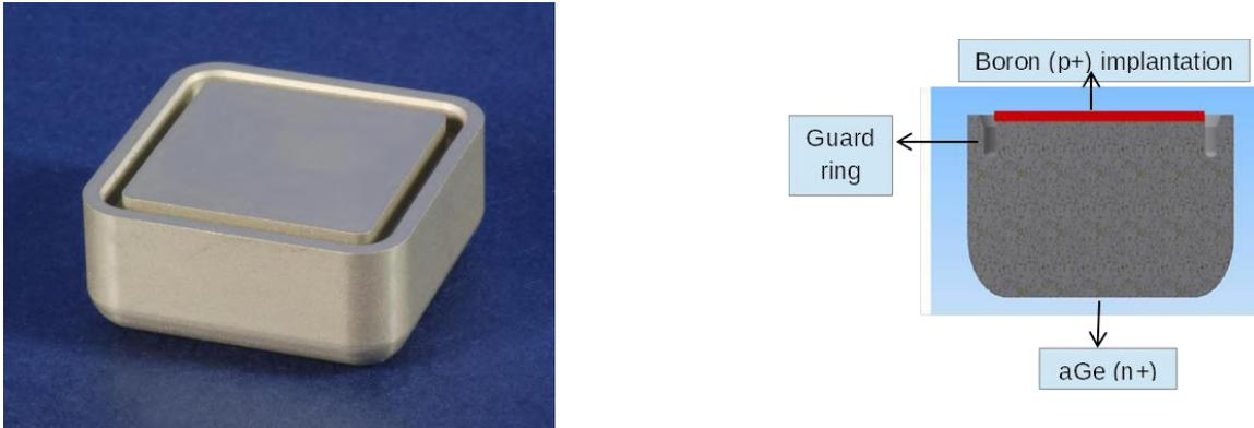
Figure 2.1: Quasi-planar prototype p-type HPGe detector with dimensions of 33.2x33.2x15.5 mm<sup>3</sup> used in order to determine the energy resolution of such a system with a single point contact read out. The depletion voltage was calculated as 450V.
