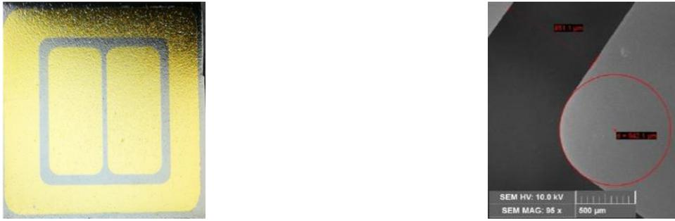
Figure 1.B.2: Photography of the segmented detector (left) and detail of the border of the segment observed by Scanning Electron Microscopy (right).
