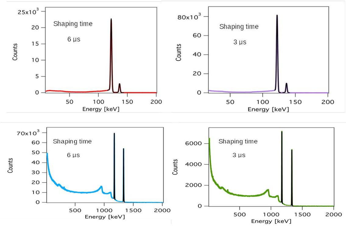
Figure 5: The observed energy spectrum with <sup>57</sup>Co source. The spectrum on the left side was recorded using a 6 μs shaping time constant while the one on the right side was obtained with a 3 μs shaping time constant.
