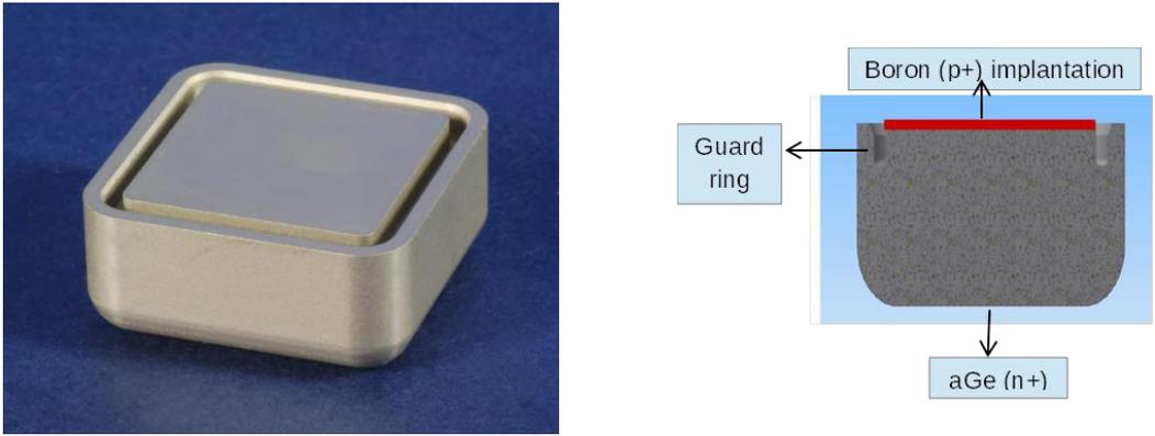
Figure 3: Quasi-planar prototype p-type HPGe detector with dimensions of  $33.2 \times 33.2 \times 15.5 \text{ mm}^3$  used in order to determine the energy resolution of such a system with a single point contact read out. The depletion voltage was calculated as 450V.
