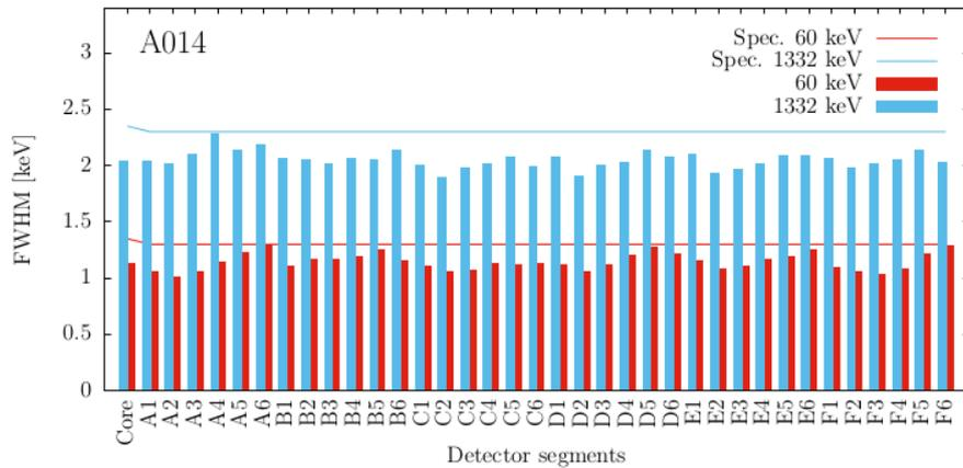
Figure 2: Energy resolution values for an encapsulated HPGe detector. Values are given for the central core contact and 36 segment signals for low energies of 60 keV and high energies of 1.3 MeV. The specifications are indicated.
