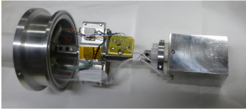
Figure 4: Semi-planar crystal placed in a POPTOP type capsule. The assembly and front-end electronics is shown.
