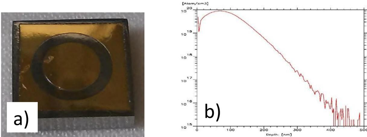
Figure 1 a) Prototype of HPGe detector with two electrically separated segments. b) Concentration profile of the ion-implanted  $^{11}\text{B}$  dopant measured by SIMS technique.
