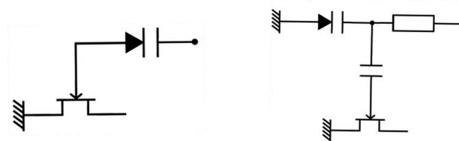
Figure 6: Different kind of couplings were used in order to read the signal at GSI and SEMIKON. Left drawing illustrates the DC coupling used at GSI and the left drawing shows the AC coupling used by SEMIKON.
